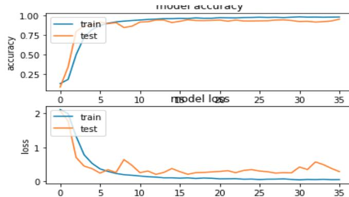
Figure 2. Validation Accuracy and Error Loss of VGG16 model
